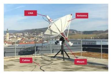
A compact radio telescope for amateur radio astronomy: the antenna installed on the equatorial mount.
