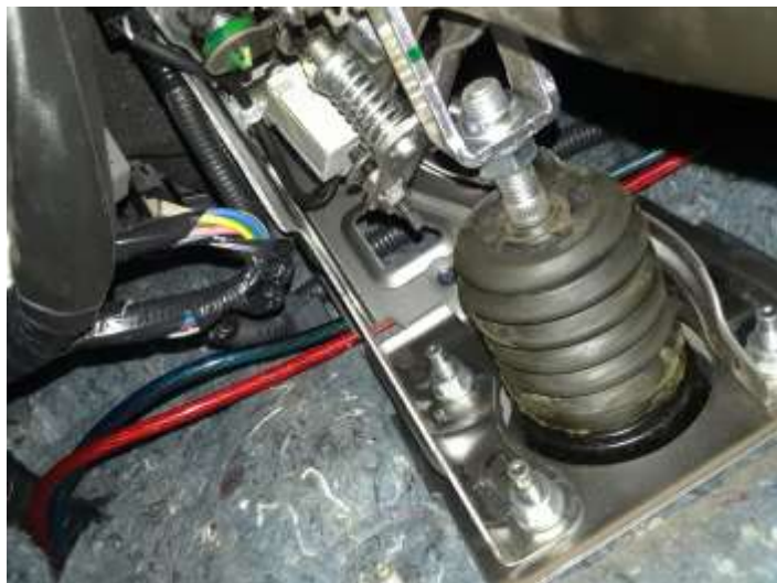
Keeping wires well out of the way of the Driver's feet
