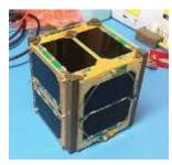
The RadFxSat-2 spacecraft bus is built on the Fox-1 series but features a linear transponder "upgrade" to replace the standard FM transponder in Fox-1A through D. In addition, the uplink and downlink bands are reversed from the previous Fox satellites in a
