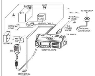
This image does not show it, but some of the instructions show the negative lead also going through the grommet, but connecting to the chassis away from the battery connection.
