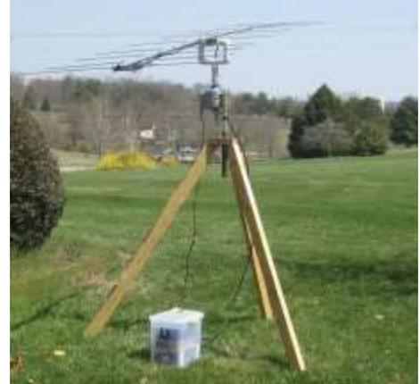
5. A Small Rotor - a TV rotor for Azimuth adjustments will suffice. You may manually adjust Elevation but it's not necessary. EME contacts can be made during the first hour after Moonrise or the last hour prior to Moonset. A Yagi pointing to the horizon will normally allow you to work EME till the Moon is up to 15 or 18 degrees above the horizon.
